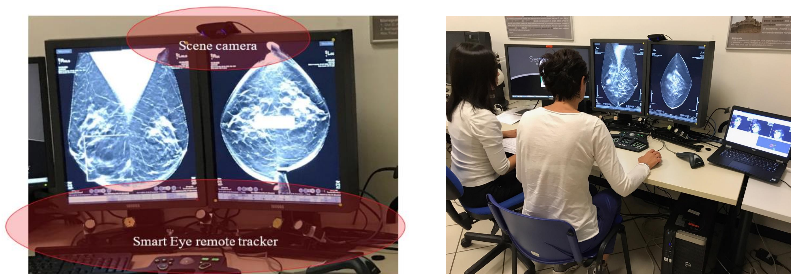
Figure 1. Left: Set up of eye tracking devices on the dual screen mammography workstation. Right: Participant is reading a DBT case while her eye movement data were collected.
