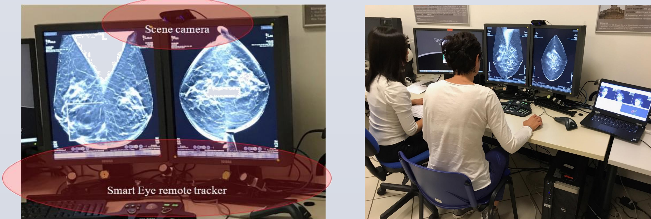
Figure 1. Left: Set up of eye tracking devices on the dual screen mammography workstation. Right: Participant is reading a DBT case while her eye movement data were collected.
